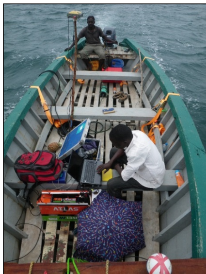
Surveying the seabed at Kilwa using the SwathPlus 468kHz bathymetric sidescan.
