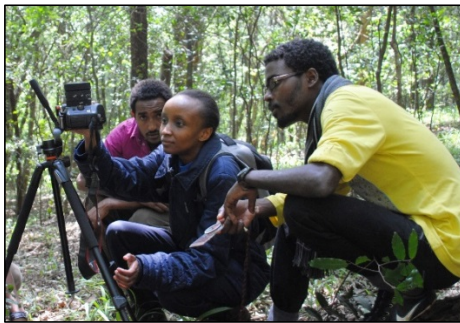
Students taking upward looking hemispherical images to estimate LAI in Karura Forest Reserve.
